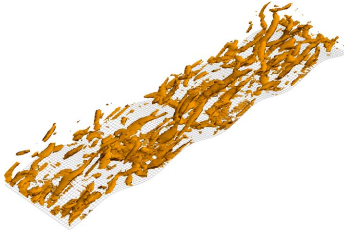
Fig. 20. Instantaneous snapshot of vortex cores plotted as isocontours of \lambda_2 = -50 in fully developed steady wavy flow with the IBM approach.
